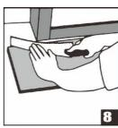
The gap between the bottom of a door and the vinyl flooring should be I cm height.
